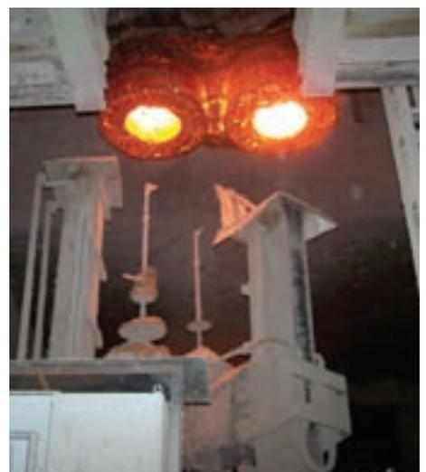
Fig 18: Gunning robot with two lances for inside and outside repair
