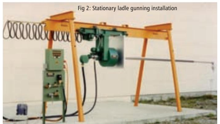
Fig 2: Stationary ladle gunning installation
