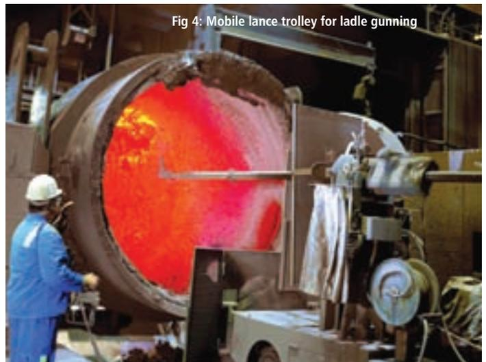
Fig 4: Mobile lance trolley for ladle gunning
