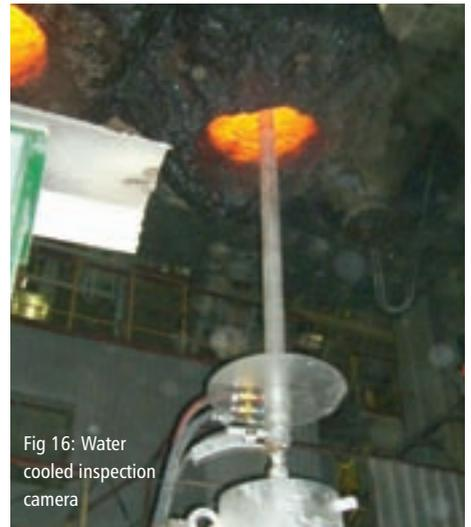
Fig 16: Water cooled inspection camera
