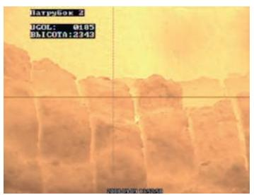
Fig 17 (left): Inside picture of RH-snorkel taken with inspection camera
